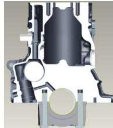
Figure 6. No. 4 main bearing and main oil channel.
